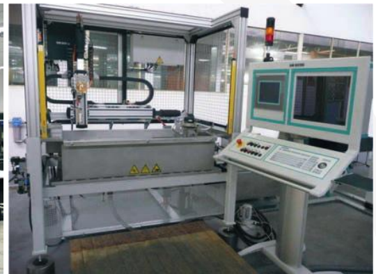
Crack detection - Ultrasonic
